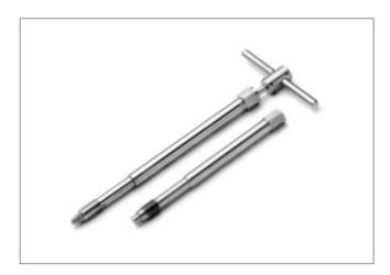
The Cleaning Tool Kit is used to remove excess plastic from transducer mounting holes prior to installation. Installation of transducers into plugged and/or dirty mounting holes is a major cause of installation-related damage. The Cleaning Tool Kit allows the mounting hole to be properly cleaned and checked for integrity.
